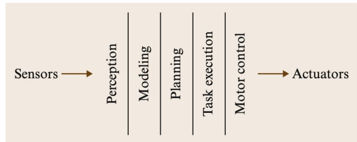
Fig. 8.2 The sense-plan-act (SPA) paradigm (after [8.3], with permission)
