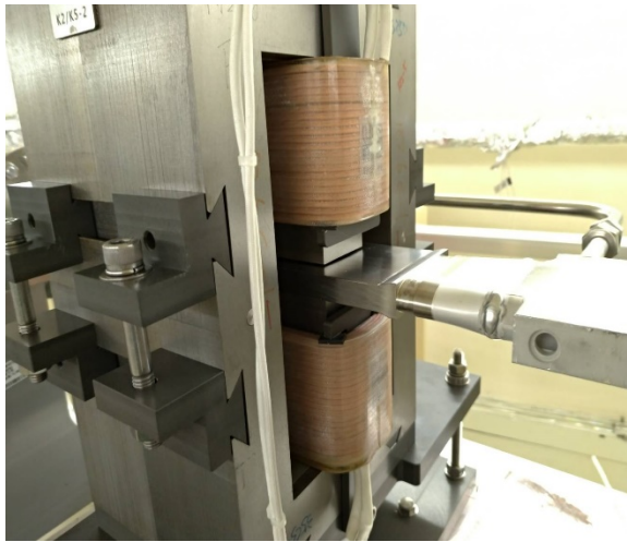
Fast switching kicker 段用鈦合金真空腔
