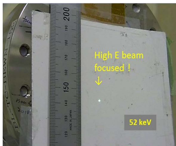
圖 2.12：SP12B：High Energy beam focused by Si220 bent monochromator
