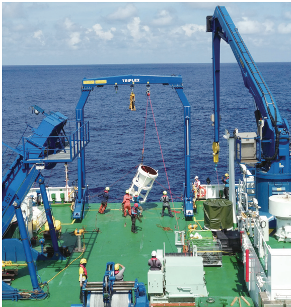
Deployment of an anchored string of deposit collector
