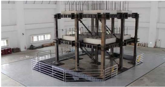
The Tainan laboratory's long stroke, high-velocity vibration system can help develop technologies to resist shaking from near-fault earthquakes.
