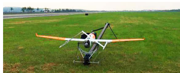
TTFRI's unmanned aerosonde aerial vehicle on its catapult in August 2017, while preparing for take-off on a mission during the approach of Typhoon Hato
